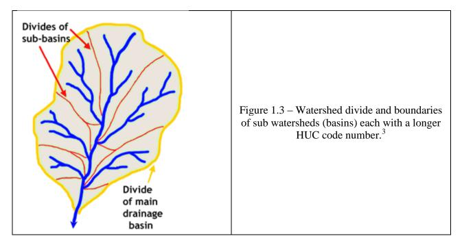
The U.S. Geological Survey (USGS) has developed another way to describe how smaller streams become larger rivers. USGS established Hydrological Unit Codes (HUCs) to delineate drainage basins at different scales, sometimes referred to as a "nesting" system (Figure 1.3. There are six different levels of units, which are arranged by size. The more digits are included in a HUC, the
